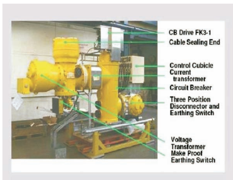
Fig. 12.1: A view of equipment of a GIS
